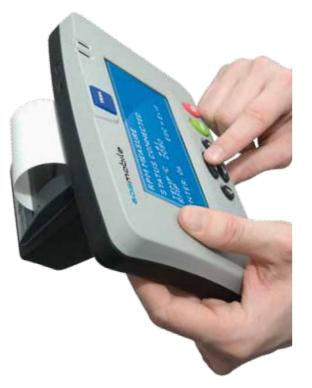
Thanks also to Bluetooth wireless data communications, TEXA exhaust gas analysis solutions can eliminate all unwanted cables around the workshop, not only between the analysers and the display units, but between the analysers and the main power supply too.
